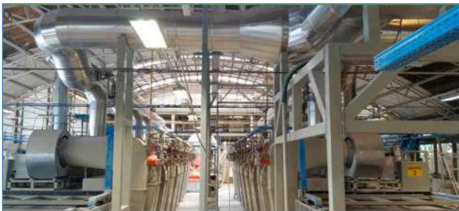
Image 7: Heat recovery from kiln to dryer at ceramics factory in Morbi Cluster
