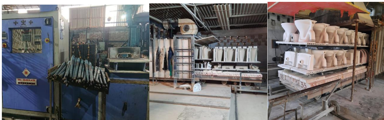
Figure 4: Induction furnace at Howrah and double decker kiln loading at ceramics factor in Thangadh
